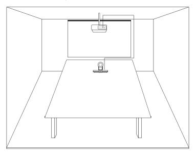
Locate the HDMI port on the VC800/VC500 codec, and connect it to the projector with the supplied HDMI cable.
