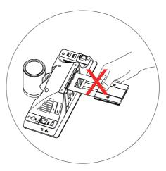
Do not pick up the bracket which connects with a VC500 codec, the VC500 codec may fall down in this situation.
