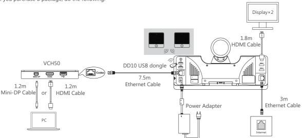
The CPW90 wireless microphones and DD10 USB dongle are automatically paired from the factory.
