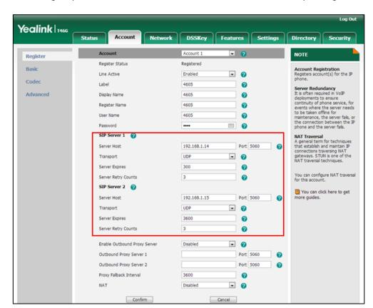
4. Configure parameters of SIP server 1 and SIP server 2 in the corresponding fields.
