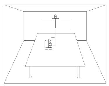
Locate the Line Out port on the VC800 codec, and connect it to the external speaker using a 3.5mm jack cable. This is not applicable to VC500 video conferencing endpoint.
