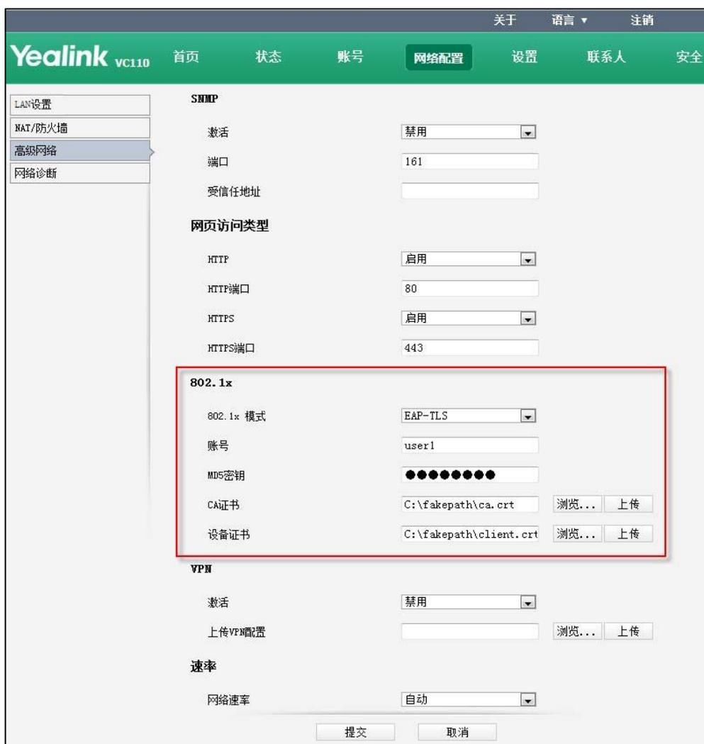
The screenshot displays the Yealink VC110 web management interface. The top navigation bar includes '关于', '语言', and '注销'. The main menu has '首页', '状态', '账号', '网络配置', '设置', '联系人', and '安全'. The left sidebar shows 'LAN设置', 'NAT/防火墙', '高级网络', and '网络诊断'. The main content area is divided into sections: 'SNMP', '网页访问类型', '802.1x', 'VPN', and '速率'. The '802.1x' section is highlighted with a red box and contains the following fields:
