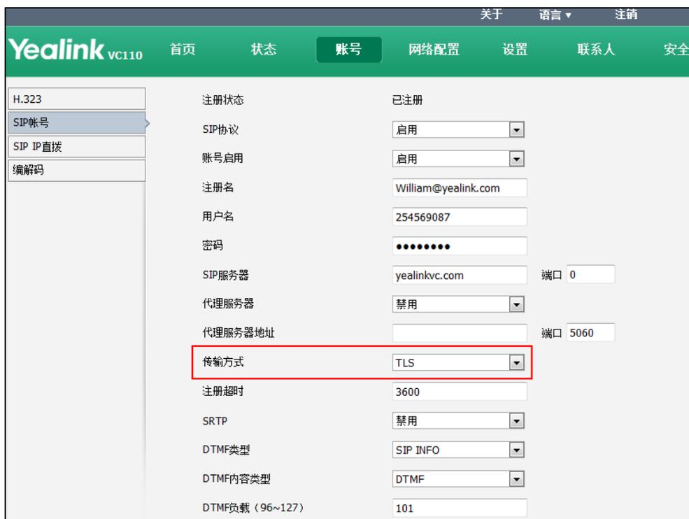
The screenshot shows the Yealink VC110 account configuration interface. The '账号' (Account) tab is selected. The '传输方式' (Transport Method) dropdown menu is highlighted with a red box and set to 'TLS'. Other configuration options include SIP protocol, account status, registration name, username, password, SIP server, proxy server, and DTMF settings.
