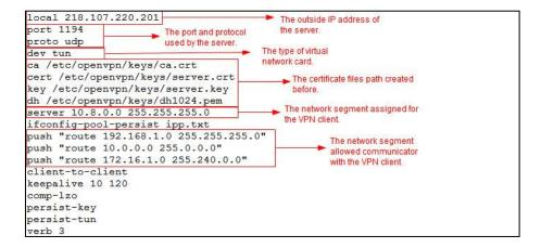
According to the actual network environment, configure the network settings of the server, such as the TCP/IP forwarding feature, Internet connection sharing feature and routing entries between the VPN clients and the Intranet. For more information, contact your network administrator.
