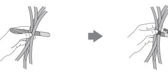
Fasten the cables with the cable tie
