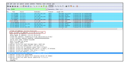
After obtaining the VLAN ID from DHCP server, IP phone will release the leased IP address (5.5.5.18) and start a new DHCP Discover message with the VLAN-tag 111.
