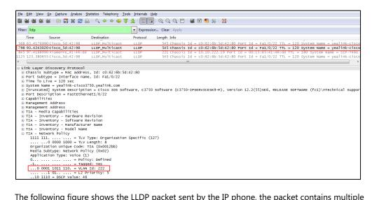
The following figure shows the LLDP packet sent by the IP phone, the packet contains multiple TLVs (after obtaining VLAN ID).
