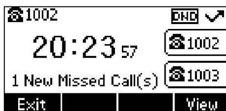
When DND feature is enabled, the IP phone supports displaying a large DND icon on the idle screen. For more information, contact your system administrator.
