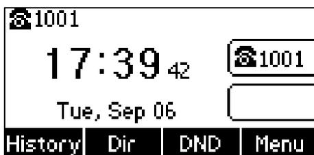
The idle screen displays the label of default account, time and date, and four soft keys.
