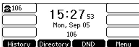
The idle screen displays the label of default account, time and date, and four soft keys.
