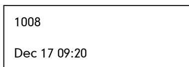
The idle screen displays the label of current account, time and date.
