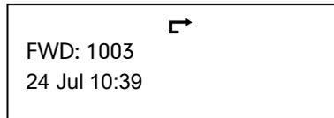
Call forward is configurable via web user interface at the path **Features->Forward & DND**.
