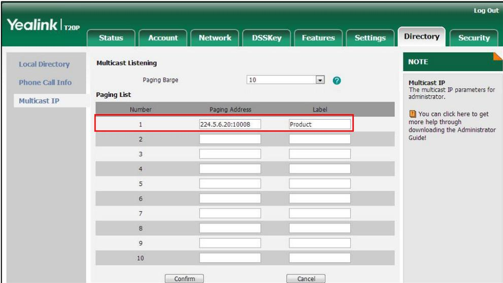
The screenshot shows the Yealink T20P web interface. The 'Directory' tab is selected, and the 'Multicast IP' sub-tab is active. The 'Multicast Listening' section shows a 'Paging Barge' dropdown set to '10'. Below it is a 'Paging List' table with 10 rows. The first row is highlighted with a red box and contains the following data:
