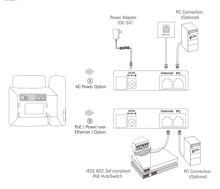
Note: PoE is only applicable to the SIP-T22P IP phone. If inline power (PoE) is provided, you do not need to connect the power adapter. Make sure the hub/switch is PoE-compliant.
