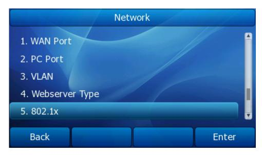
2) Set "802.1x Mode" to be "EAP-MD5", fill in the correct Identity and MD5 password, press the "save" button;
