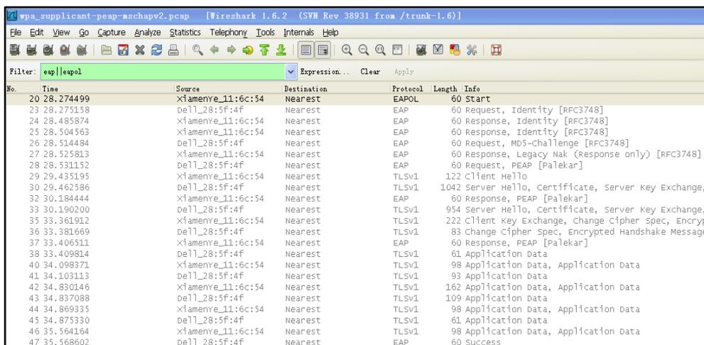
The following screenshot of the Wireshark shows a sample of a successful authentication process using EAP-TTLS/EAP-MSCHAPv2 protocol:
