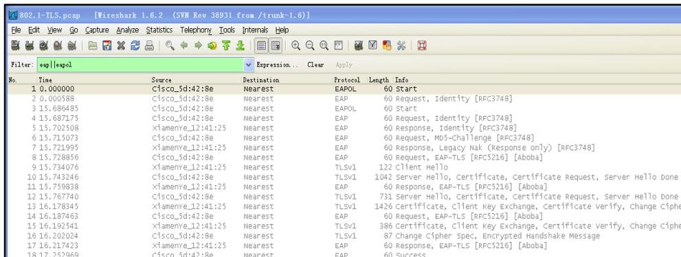
The following screenshot of the Wireshark shows a sample of a successful authentication process using PEAP-MSCHAPv2 protocol:
