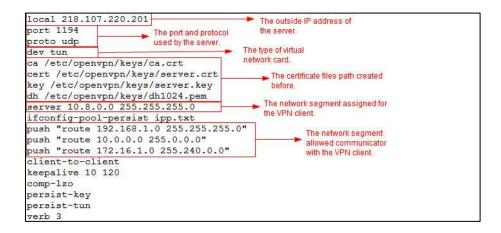
According to the actual network environment, configure the network settings of the server, such as the TCP/IP forwarding feature, Internet connection sharing feature and routing entries between the VPN clients and the Intranet. For more information, contact your network administrator.
