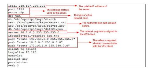
According to the actual network environment, configure the network settings of the server, such as the TCP/IP forwarding feature and routing entries between the VPN clients and the Intranet. For more information, contact your network administrator.
