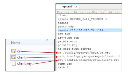
Ensure that the following configurations in the server configuration file and client configuration file are exactly matched.
