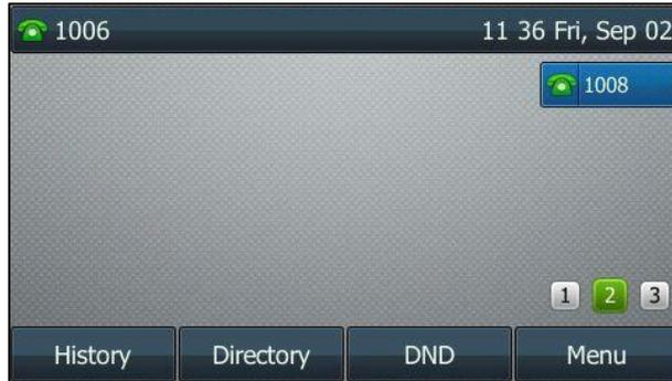
The line key in the right bottom is used to switch pages.
