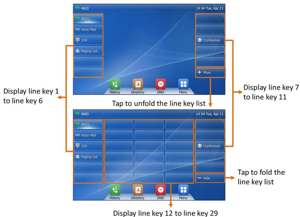
The Line Key screen on the SIP-T48S/T48G IP phone is shown as below:
