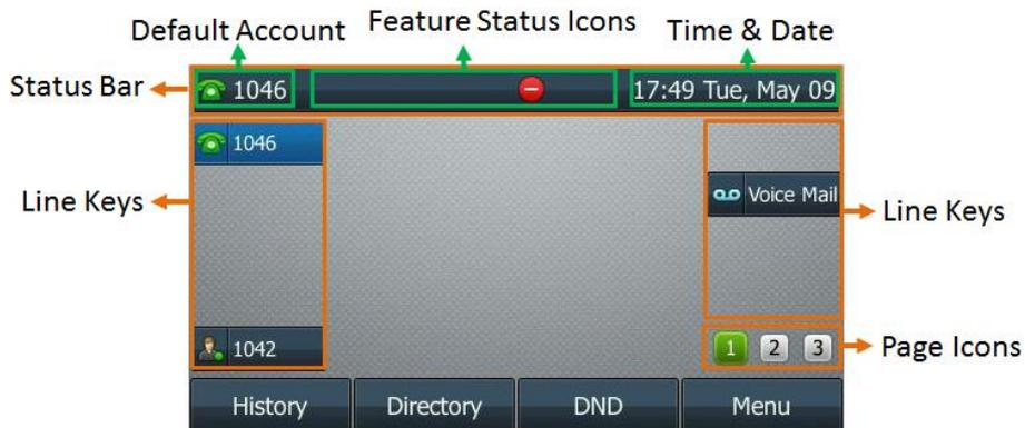
For SIP-T42S/T42G/T41S/T41P IP phone, the page icons appear only when you assign functionality to line key located in line key 7-15, refer to [DSS Keys](#) for more information. The Idle screen on SIP-T42S/T42G/T41S/T41P IP phone is shown as below:
