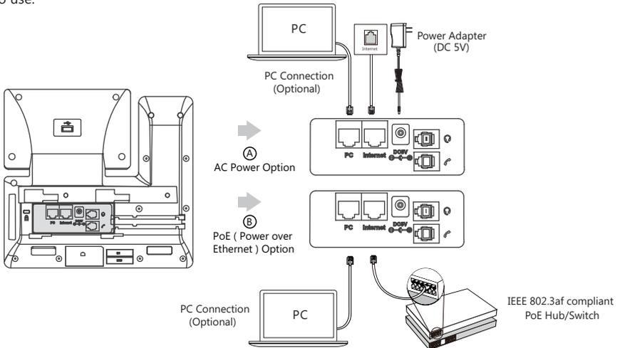
**Note:** The IP phone should be used with Yealink original power adapter (5V/2A) only. The use of the third-party power adapter may cause the damage to the phone. If you are connecting a PC to your phone, we recommend that you use the Ethernet cable provided by Yealink. If inline power (PoE) is provided, you don't need to connect the power adapter. Make sure the hub/switch is PoE-compliant.
