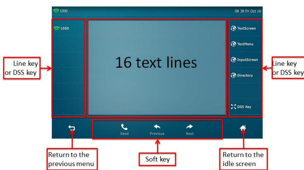
**The LCD screen and keys available for XML applications on a Yealink SIP-T57W/T48U/T48G/T48S IP phone are:**
