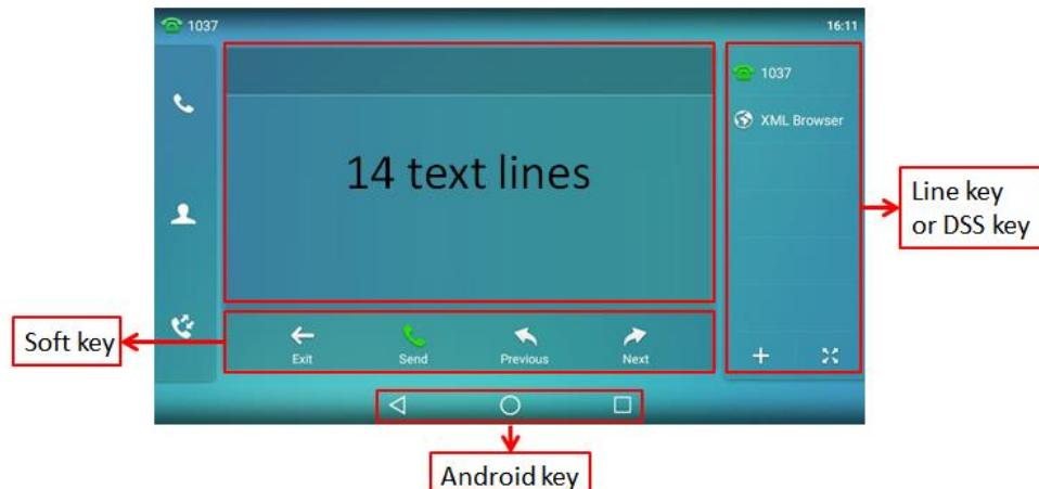
**The LCD screen and keys available for XML applications on a Yealink SIP VP-T49G IP phone are:**
