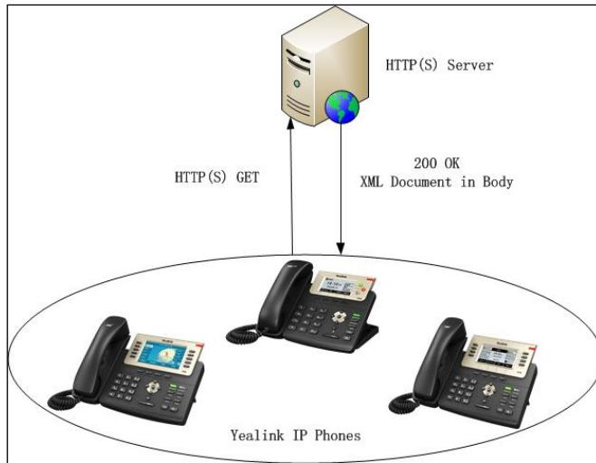
Figure1 Yealink IP phone acting as a client
