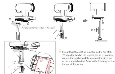
Choose the following installation method when the thickness of the TV is between 50mm and 100 mm.
