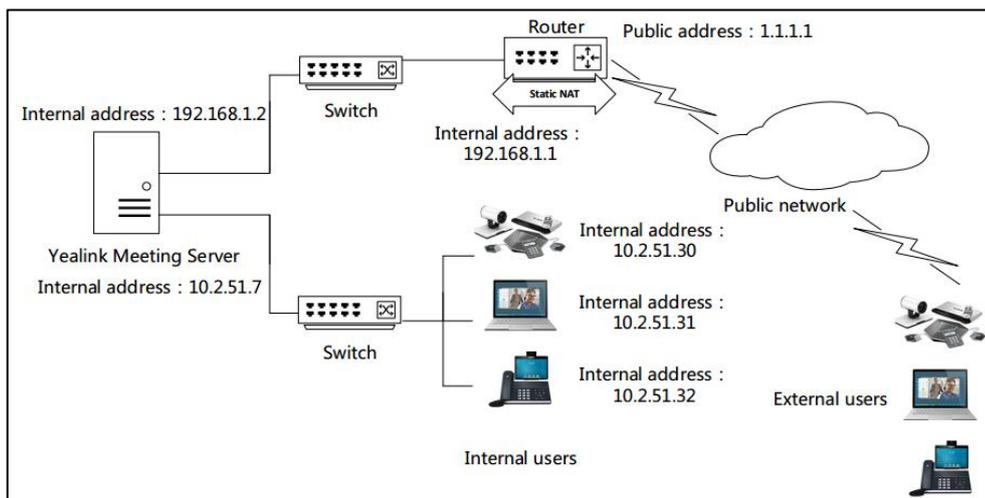
**To configure internal and external network settings via YMS:**
