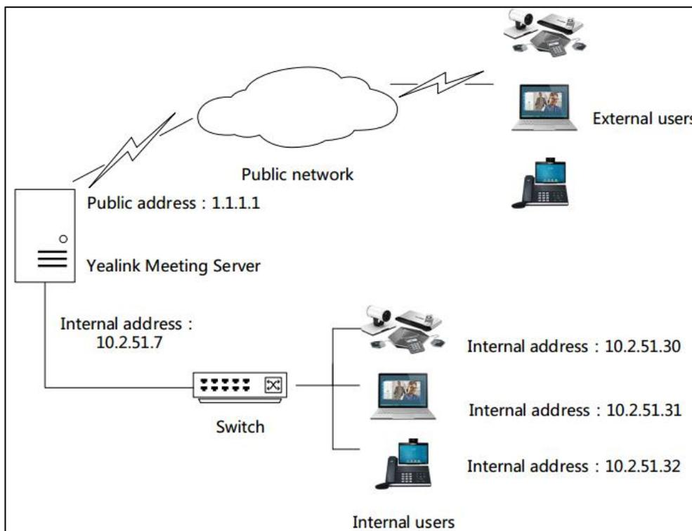
**To configure internal and external network settings via YMS:**
