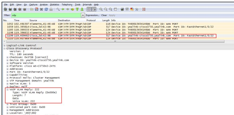
The following figure shows the CDP packet sent by the IP phone (after obtaining VLAN ID-without VLAN Query field).
