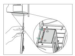
If your endpoint cannot be mounted on the top of a TV when the bracket has reached the given location, you should remove the bracket, and then convert its direction. Refer to the following section for more information.
