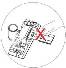
Do not pick up the bracket which connects with an endpoint, the endpoint may fall down in this situation.
