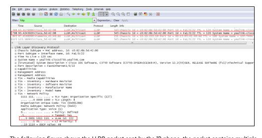
The following figure shows the LLDP packet sent by the IP phone, the packet contains multiple TLVs (after obtaining VLAN ID).
