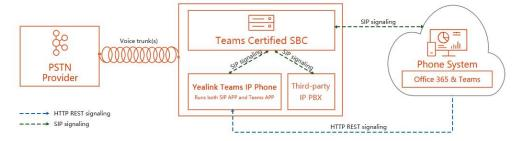
SBC can also be installed on the local virtual machine or Microsoft Azure. This document focuses on the configuration steps of installing VE SBC on the local VMware virtual machine, see <a href="Steps for AudioCodes SBC">Steps for AudioCodes SBC</a>
