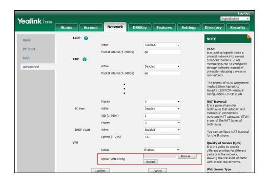
6. In the VPN block, select **Enabled** from the pull-down list of **Active**.
