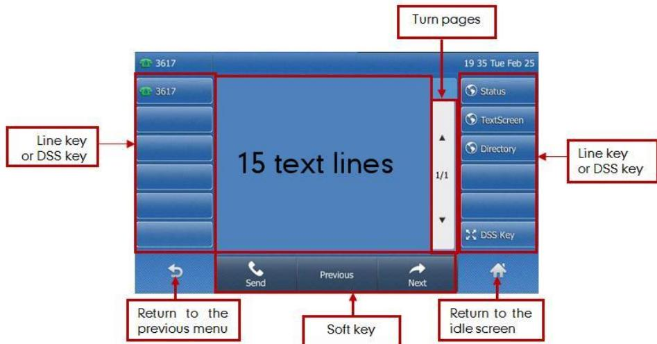
**The LCD screen and keys available for XML applications on a Yealink SIP-T46U/T46G/T46S/T29G IP phone are:**
