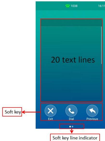
**The LCD screen and keys available for XML applications on a Yealink VP59/SIP-T58A IP phone are:**
