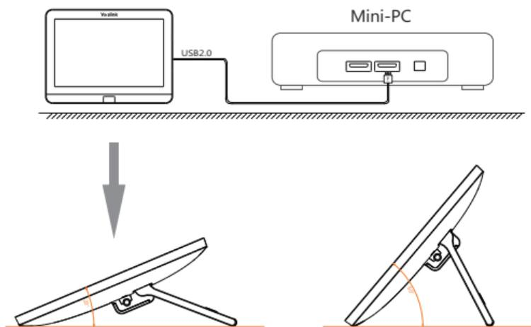
The stand can be adjusted from 23 to 50 degrees.
