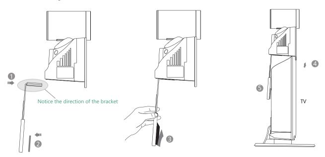
Steps: • Push the bracket along the track of the endpoint to an appropriate location.
