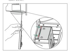
If your endpoint cannot be mounted on the top of a TV when the bracket has reached the given location, you should remove the bracket, and then convert its direction. Refer to the following section for more information.
