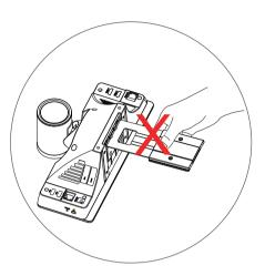
Do not pick up the bracket which connects with an endpoint, the endpoint may fall down in this situation.
