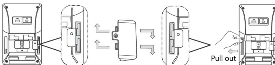
Connecting two expansion modules on a single host phone is shown as below:
