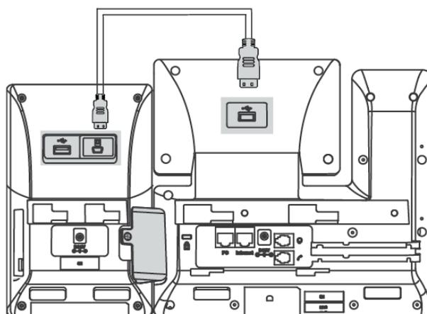
If you connect two expansion modules, connect the USB jack on the prior expansion module and the mini USB jack on the next expansion module using another supplied cable. Connecting two expansion modules on a single host phone is shown as below:
