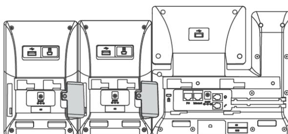
4. Connect the USB jack on the host phone and the mini USB jack on the expansion module using one supplied cable.
