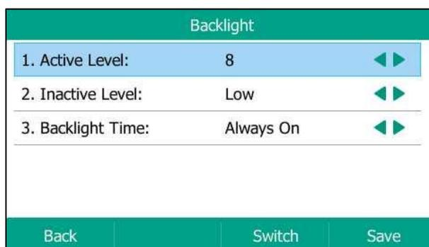
2. Press **◀** or **▶**, or the **Switch** soft key to select the desired level from the **Active Level** field on the host phone.
