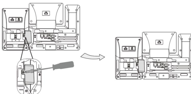
If you want to connect two or more expansion modules, pull out the silica gel and connect two expansion modules as below.
