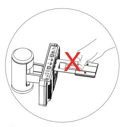
Do not pick up the bracket which connects with a system, the system may fall down in this situation.
