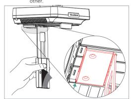
If your system cannot be mounted on the top of a TV when the bracket has reached the given location, remove the bracket, and then convert its direction. Refer to the following section for more information.
