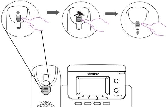
The hookswitch tab has a lip which allows the handset to stay on-hook when the IP phone is mounted vertically.
