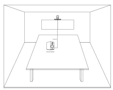
Locate the Line Out port on the VC800 codec, and connect it to the external speaker using a 3.5mm jack cable.
