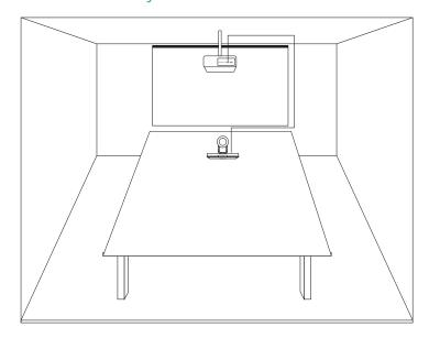
Locate the HDMI port on the VC800 codec, and connect it to the projector with the supplied HDMI cable.
