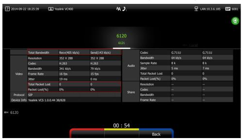
If total packet loss or packet loss rate is high, it is recommended that you check the causes of this problem.
