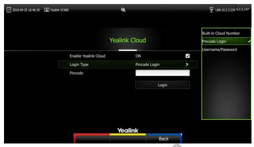
After successful registration, the display device displays , and the LCD screen of the video conferencing phone displays .
