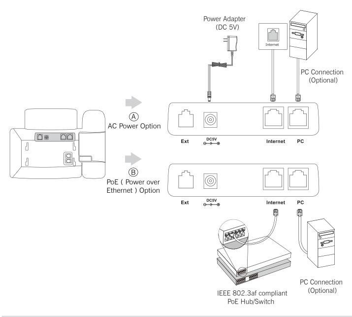
Note: If inline power (PoE) is provided, you do not need to connect the power adapter. Make sure the hub/switch is PoE-compliant.
