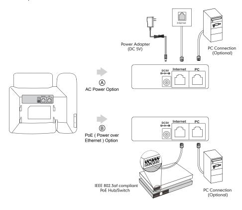
Note: PoE is only applicable to the SIP-T21P IP phone. If inline power (PoE) is provided, you don't need to connect the power adapter. Make sure the Etherne cable and hub/switch are PoE compliant.
