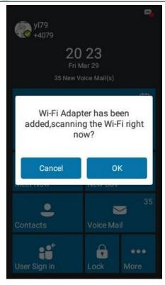
If the phone is connected to the wired network and the Wi-Fi mode is also activated, the phone will use the wireless network by default. If there is no available wireless network, the phone will use the wired network instead automatically.
