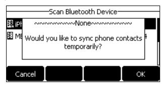
**5.** (Optional.) Press **OK** to enable the mobile contacts sync feature and the IP phone will sync the mobile contacts temporarily, or press **Cancel** to disable mobile contacts sync feature and the IP phone will not sync the mobile contacts.
