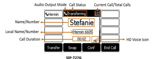
When you are during a call, press the OK key to view the current time & date and the phone status (not applicable to SIP-T19(P) E2/T21(P) E2/T29G IP phones), the screen on the IP phone is shown as below:
