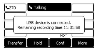
During a recording, if there is insufficient free space (30 minutes or 10 minutes left) on the USB flash drive, the IP phone will prompt you a message (XX minutes left for call recording). If no free space on the USB flash drive during recording, recording is stopped and saved in the USB flash drive automatically.
