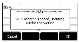
You can press **OK** to activate Wi-Fi mode directly and to scan Wi-Fi devices automatically.
