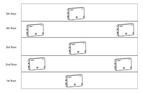
• If the degree of attenuation of the building construction materials (e.g., metal) of the building is high, follow the above introduced steps (single floor) to deploy each floor as individual parts. For more information, refer to Deployment in a Single Floor Building.
