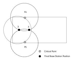
**5.** Follow the above steps to locate area centers for other base stations. Once identified, place the deployment base station at intersection points where each of the coverage cells crossed during deployment. Verify the coverage cells that reach all areas expected.
