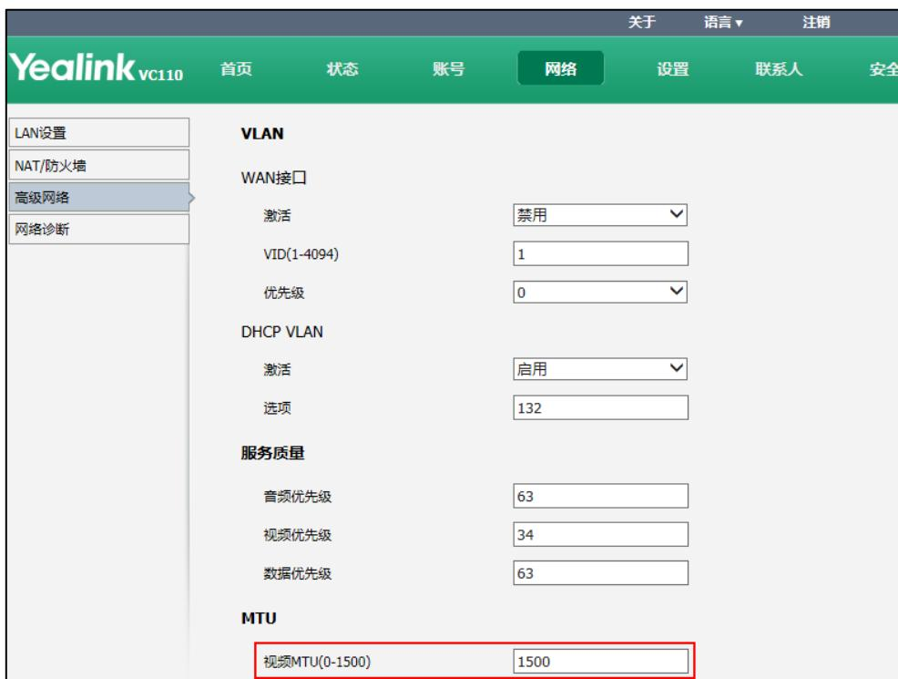
The screenshot shows the Yealink VC110 network configuration interface. The left sidebar has a menu with options: LAN设置, NAT/防火墙, 高级网络 (highlighted in blue), and 网络诊断. The main content area has tabs for VLAN, WAN接口, DHCP VLAN, 服务质量, and MTU. In the MTU tab, there is a field labeled "视频MTU(0-1500)" with the value "1500". This field is highlighted with a red rectangle.
