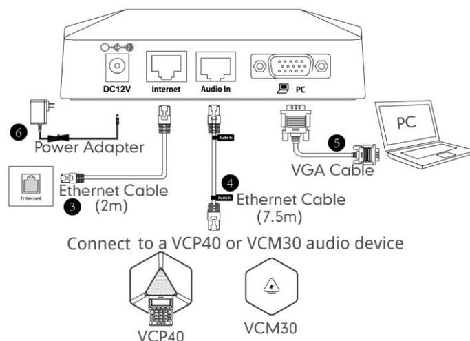
You can fasten all cables with cable ties after all devices are connected.
