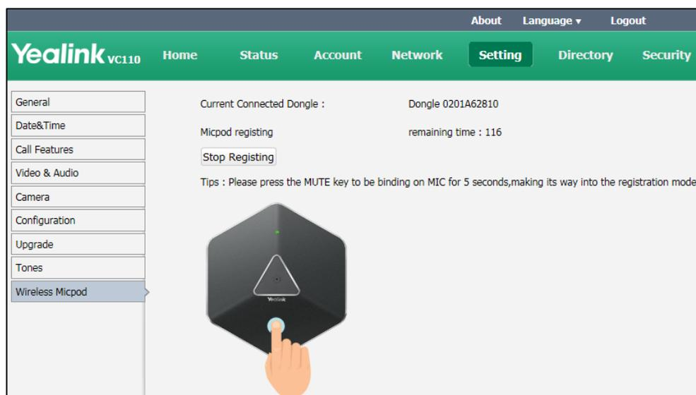
3. Tap and hold the mute button on the VCM60 video conferencing wireless microphone for 5 seconds until the mute indicator LED flashes orange. The VCM60 video conferencing wireless microphone and the dongle will be paired automatically. If this fails, the VCM60 will exit registration mode in 2 minutes.
