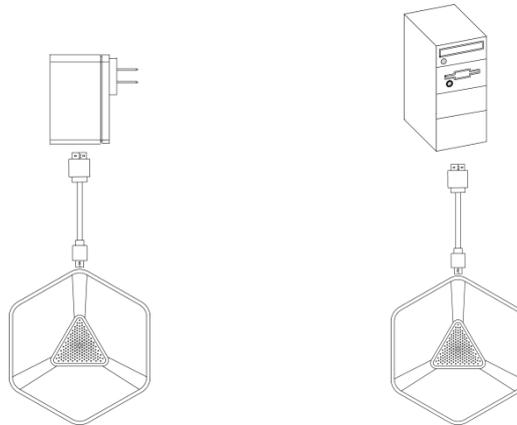
The VPM60 can work normally during charging. If you charge the VCM60 when it is working, the display device prompts “The battery is charging!”, and the
