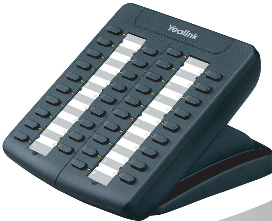
Yealink EXP38 Expansion Module is designed for improving the power and flexibility of Yealink advanced IP phones SIP-T28P & SIP-T26P. It features 38 fully programmable DSS keys each with a dual-color LED, connected to and controlled by the IP Phone with an RJ-12 cable line. It creates up to 228 additional programmable extensions when 6 EXP38 are daisy chained with the IP Phone.
