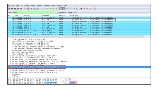
The following figure shows the DHCP message received by the IP phone (DHCP server sent the ACK message to the phone):
