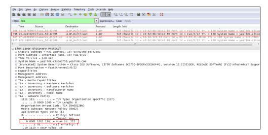
The following figure shows the LLDP packet sent by the IP phone, the packet contains multiple TLVs (after obtaining VLAN ID).
