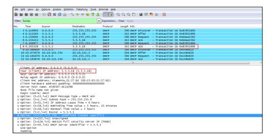
After obtaining the VLAN ID from DHCP server, IP phone will release the leased IP address (5.5.5.18) and start a new DHCP Discover message with the VLAN-tag 111.
