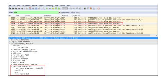
The following figure shows the CDP packet received by the IP phone (with VLAN Reply field).
