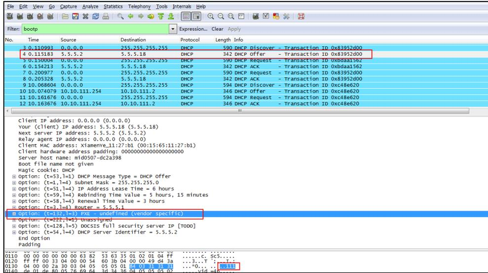
The following figure shows the DHCP message received by the IP phone (DHCP server sent the ACK message to the phone):
