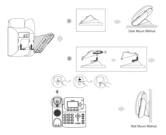
**Note** The hookswitch tab has a lip which allows the handset to stay on-hook when the IP phone is mounted vertically.
